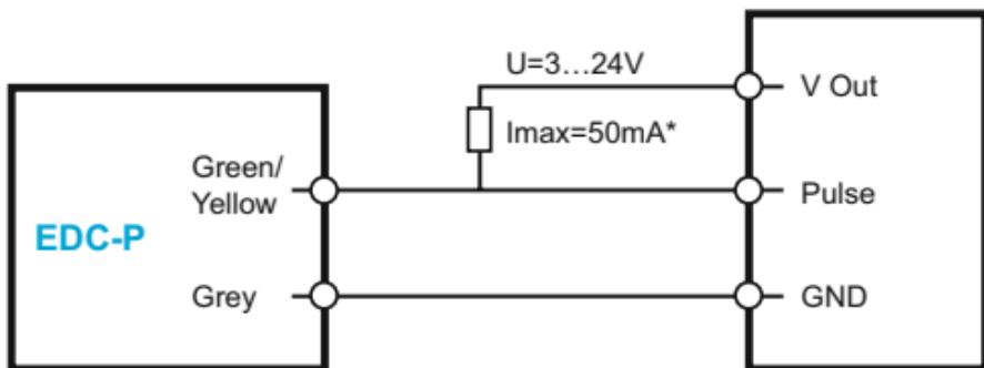
\* The connection of an external resistor may be necessary to ensure the current limiting.
